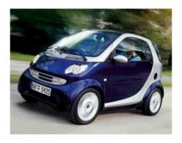
The Smart Car is one of the most energy efficient vehicles in this country. It gets its fuel economy without using complex hybrid technology, but rather by reducing the vehicles weight and aerodynamic drag. Smart Car drivers are making a statement everywhere they drive that you don't need an SUV to drive around a city. This is an important message and a great battle was won by successfully importing this car.
